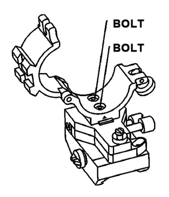
CONNECT THE HOLDING MOUNT WITH THE BOTTOM MOUNT BY TWO BOLTS, THE SYMBOL AT BOTTOM OF THE HOLDING MOUNT IS AS THE FIGURE
